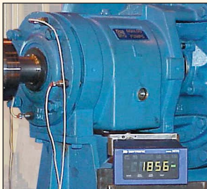
Bearing Load Measured on Test
