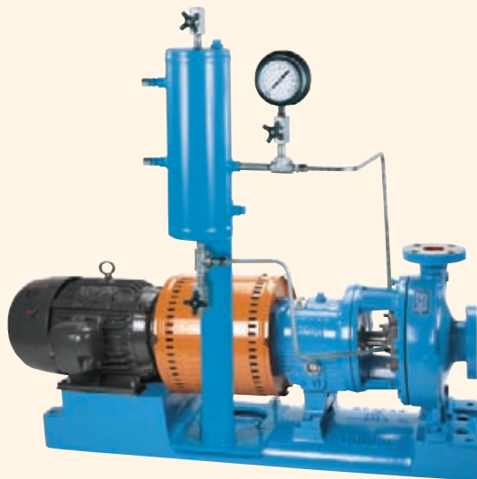
CPI PLAN 7353 Pressurized circulation lubricates double seal faces.
