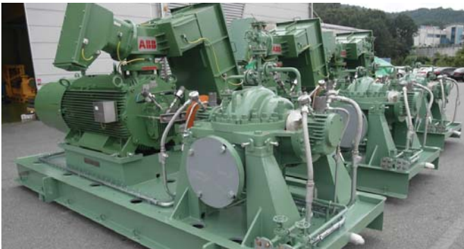
Refinery in UAE - centerline mount for higher temperatures
