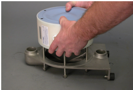
Remove the center block [16] by gently pulling apart.
