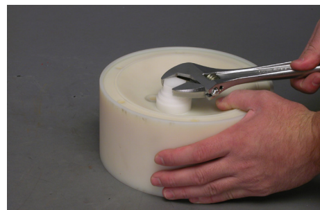
To remove the air control system, screw off both end caps using the plastic mounting tool delivered with the pump. Take out main and pilot piston.
