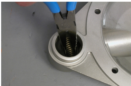
Remove the valve stops [3] and the ball valves [15] out of the side housings [1]. For the G125 and G200 the use of a screwdriver to remove the valve stops maybe is more convenient.
