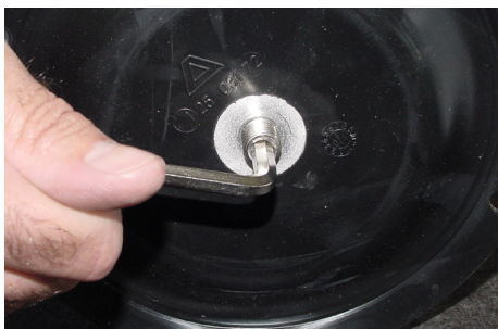
Screw out the set screws, shaft [13a].
