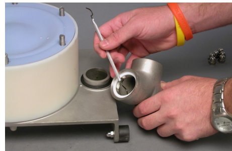
Draw the O-rings port outside [7] off the side housings [1]. Remove the inner O-rings [6] out of the ports [2].
