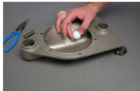
Remove the valve stops [3] and the ball valves [15] out of the side housings [1]. For the G125 and G200 the use of a screwdriver to remove the valve stops maybe is more convenient.
