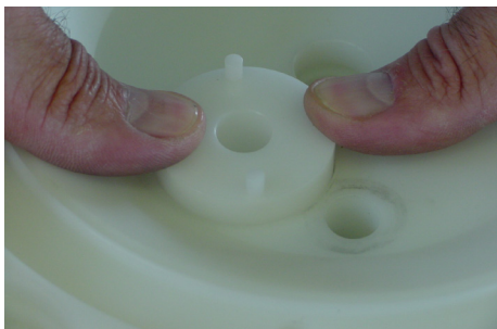
Push out the air-valve housing with the mounting tool turned around.
