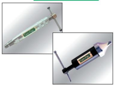
The **TP-8100** or **TP-8200** Linear Loaders™ can "reseal" the stuffing box while the machinery is in operation by injecting sealing compound with a quick turn of the handle.
