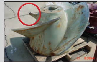
○ Broken Impeller Vanes
