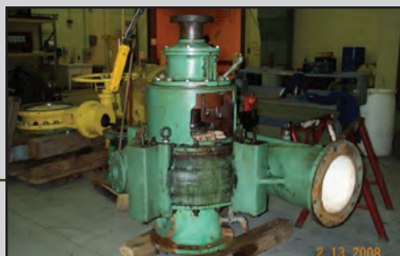
Fairbanks Morse - 50 year old obsolete pump replaced and performance restored. No expensive modifications to piping or foundations required.
