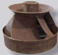
Old worn impeller
