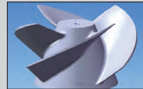
Broken Impeller is laser scanned to create a 3D model; missing vane is reconstructed.
