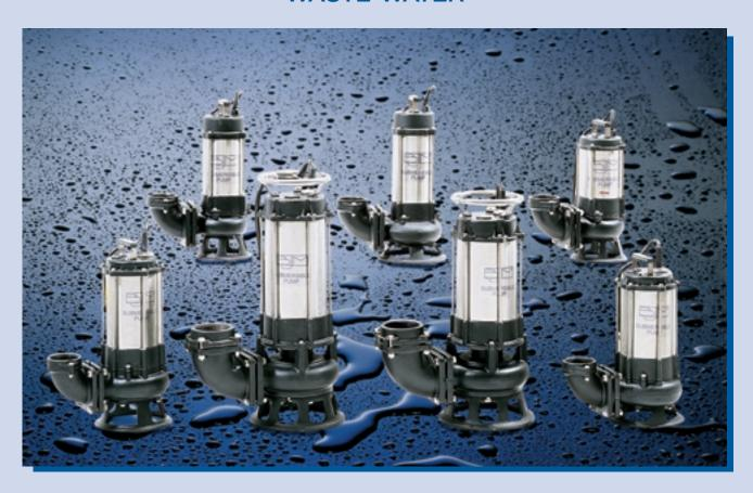
The S and SK models offer high quality and performance for a very modest investment. The pumps are equipped with motor overload protection and dual mechanical seals. The lower seal is made of Silicon Carbide. This assures longer life, less maintenance, and less down time. Each pump is tested at the factory for performance and safety.
