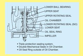
The Shredder (SK) type pumps leave solids slightly larger than if passed through a grinder pump. The shredding action is caused by using a cutting type impeller with a Tungsten Carbide Tip, against a "spiral" shaped diffuser plate.
