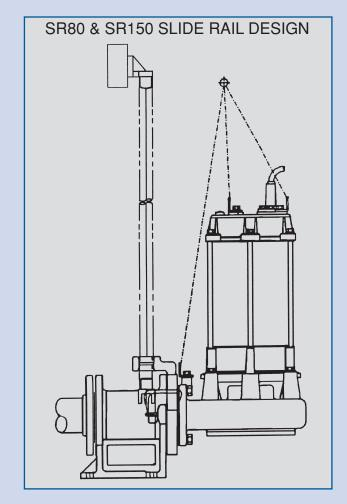
OUTSTANDING FEATURES FOR ALL BJM PUMPS: To ensure longer life, less maintenance and less downtime, BJM pumps (0.5 H.P. and up) feature double mechanical seals in a separate oil chamber. In addition, an oil seal ring has been installed under the oil chamber.
