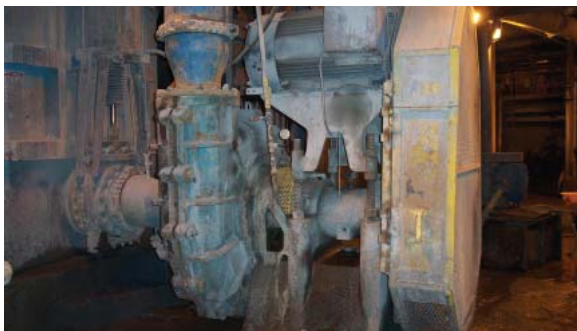
SRL-XT 14×12–36 on Ball Mill Discharge Service
