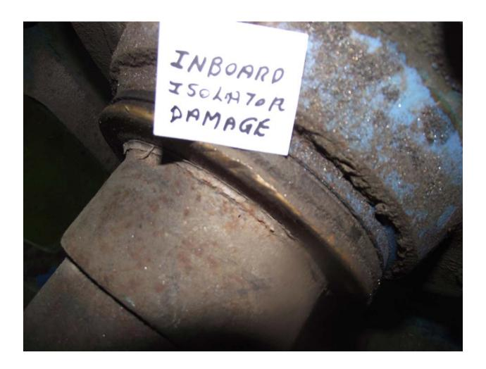
The shaft broke in operation in 2007. It has eroded to the point that shaft replacement is required this year. The depth of the wear is in excess of 1/4" (1/2" total on a 4" diameter shaft).
