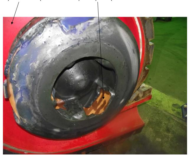
The inboard isolator is damaged and requires replacement in order to affect a proper repair and to prevent the oil from being contaminated in operation.
