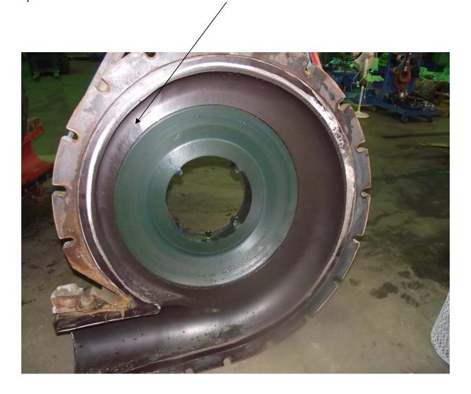
The gland side liner was also replaced in September 2009 and is in good condition. However the impeller which has portions eroded away will required repair.
