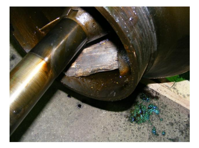
The wood found in the impeller did not damage the impeller in any way. The shaft has minimal wear at the bearing however this area will be chromed and ground to size.
