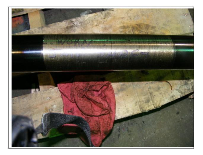
The impeller shaft is worn at the bearing. This area will be built up with chrome to the OEM specifications.
