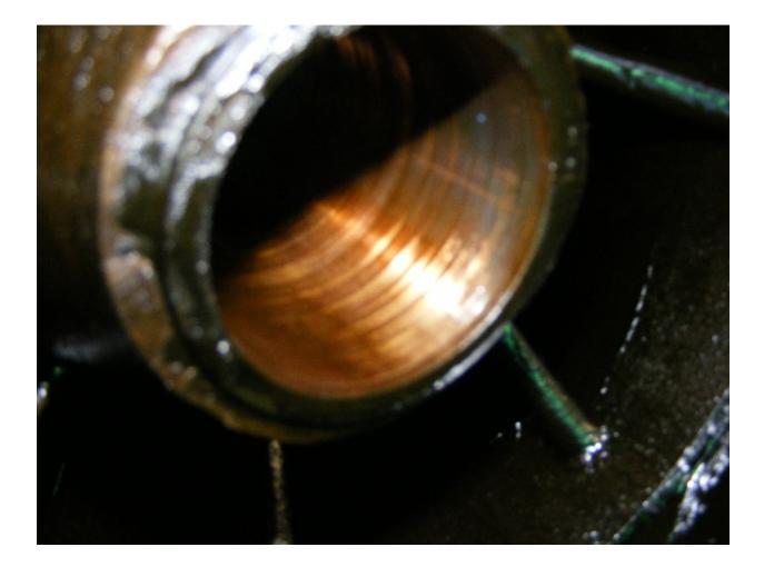
Line shaft bearing wear prevented an accurate measurement
