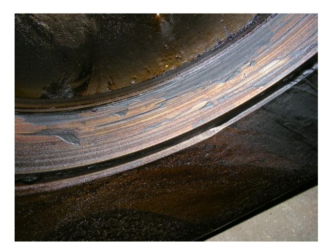
This photo shows the wear at bell suction were it comes into contact with impeller.
