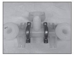
STEP 5 Remove the "Suction Manifold".
