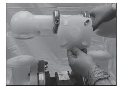
STEP 2 Remove the "Discharge Manifold".
