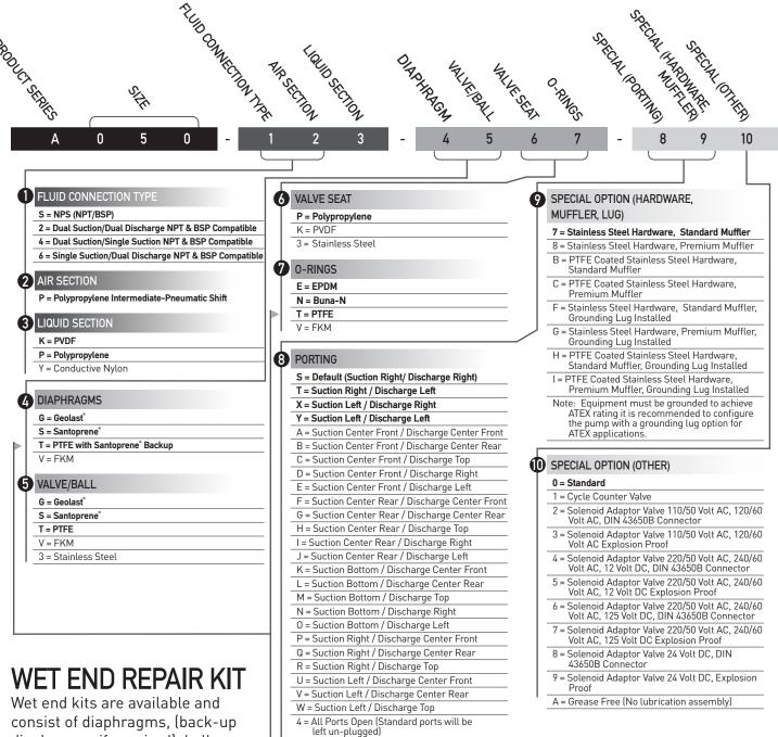
Wet end kits are available and consist of diaphragms, (back-up diaphragms if required), balls, seats and seat O-Rings.
