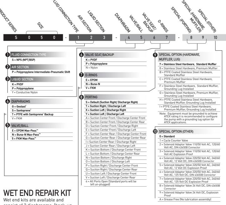
Wet end kits are available and consist of 2 diaphragms, (back-up diaphragms if required), 4 MaxPass™ valves and 4 seat 0-Rings.
