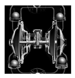
The air-valve directs pressurized air behind the left diaphragm, causing the left diaphragm to move outward (to the left).
