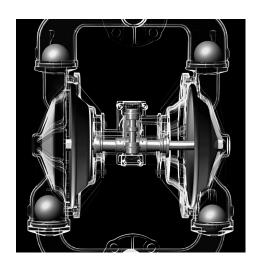
The air-valve directs pressurized air behind the diaphragm on the right, causing the diaphragm on the right to move outward (to the right).
