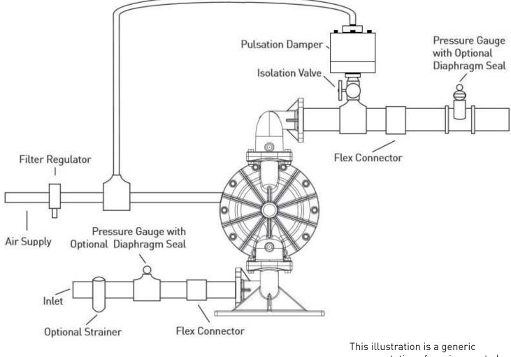
representation of an air operated double-diaphragm pump.
