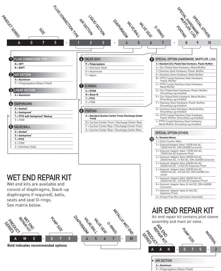
\* Solenoid Adaptor Valves only available on select pump models with polypropylene intermediate
