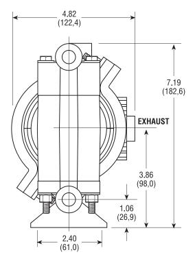
NOTE: AIR INLET IS ON THE SIDE WITH STAINLESS STEEL INSERT. THE AIR VALVE ASSEMBLY IS ON THE OPPOSITE SIDE OF THE PUMP.
