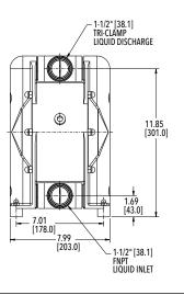
Max. Flow Rate: 40 gpm (150 lpm)
