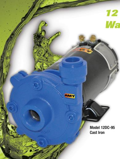
Washdown pumps are designed for OEM, chemical processing septic service, pumper and marine applications requiring a DC motor. The motor has a one hour duty rating and is furnished with a stainless steel shaft. This washdown duty pump is available in a variety of construction and seal materials to meet your specifications. Pull-from-rear design for easy servicing without disturbing any piping. Stainless Steel impeller maximizes performance. Pumps are not self-priming and require flooded suction.
